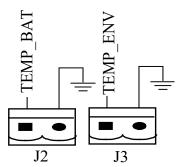
Fig.2-15 J2 and J3 for temperature detecting
