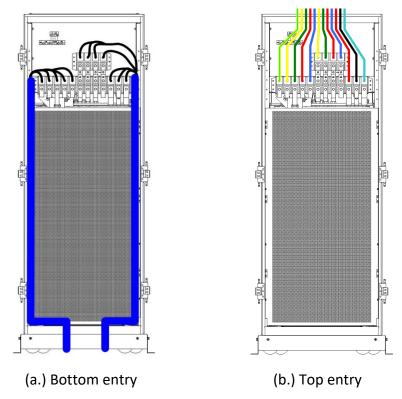
Fig.2-10 Cable entry for 6-slot cabinet
