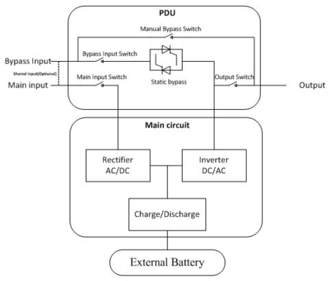
Fig.1-2 20-slot UPS Configuration
