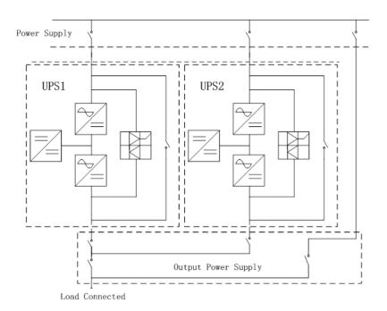
Fig. 4-6 Parallel diagram
