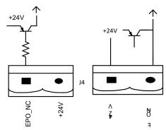
Fig.2-16 Diagram of input port for remote EPO
