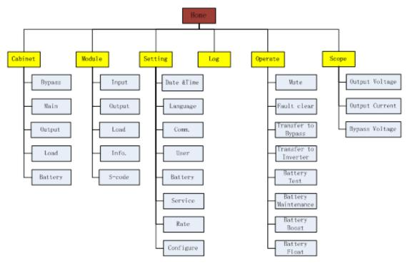
Fig.3-5 Structure of menu tree
