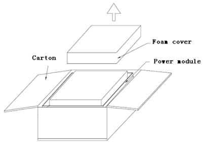
Fig.2-7 Remove the foam cover
