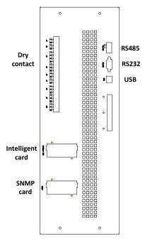
Fig.2-17 Dry contact &communication interface for 20-slot cabinet
