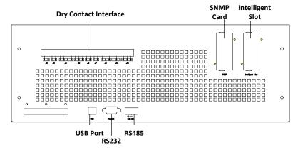
Fig.2-16 Dry contact &communication interface for 6-slot and 10-slot cabinet
