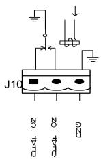
Fig.2-21 Utility failure warning dry contact interface diagram
