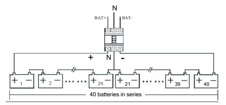
Fig. 2-9 Battery string wiring diagram
