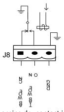
Fig.2-19 Battery warning dry contact interface diagram
