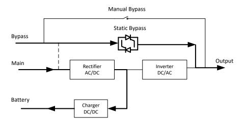
Fig.1-8 ECO Mode operation diagram
