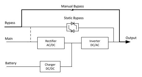
Fig.1-7 Maintenance mode operation diagram
