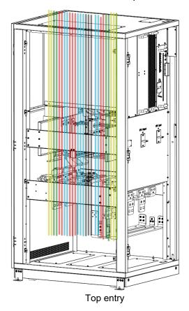
Fig.3-12 Cable entry for 20-slot cabinet
