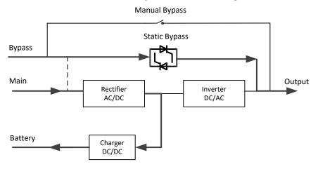
Fig.1-6 Bypass mode operation diagram
