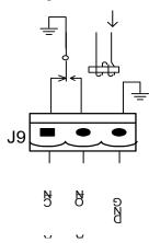
Fig.2-20 Integrated warning dry contact interface diagram
