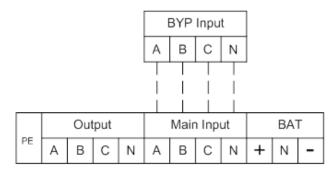
Fig.2-13 6-slot connections terminals
