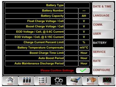
Fig.5-2 Configuration through LCD control panel
