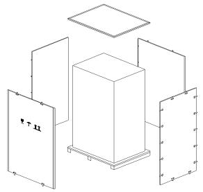
Fig.2-3 Disassemble the case
