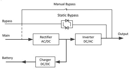
Fig.1-4 Normal mode operation diagram
