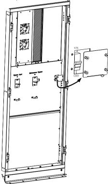
Fig.5-1 the position of Inner Control Neutral cable
