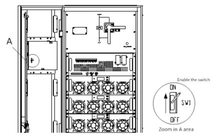
Fig.4-3 Enable the switch
