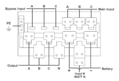
Fig.2-14 10-slot connections terminals
