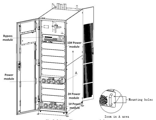
Fig.2-9 Installing power module
