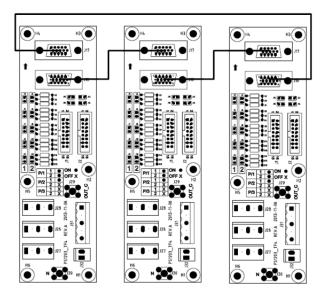
Fig.4-8 Parallel connection
