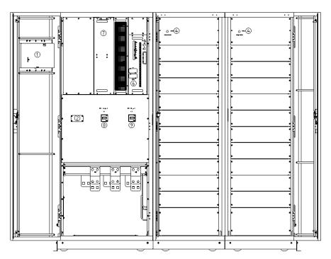
Fig. 1-14 Front view of 20-slot UPS
