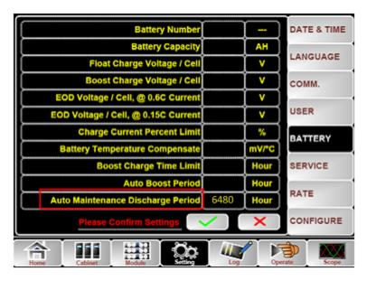
Fig.4-5 Setting period for battery auto discharge
