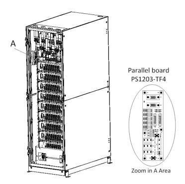
Fig.4-7 Location of the Parallel board
