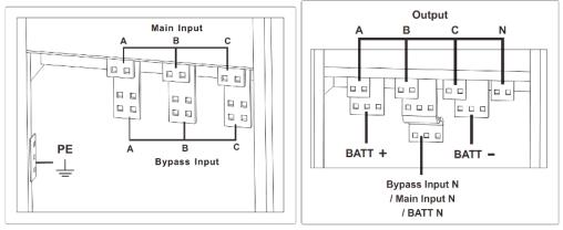
Fig.2-15 20-slot connections terminals
