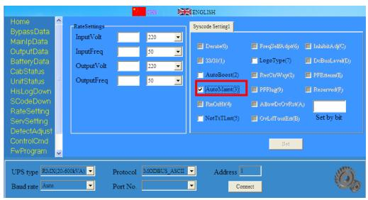
Fig.5-5 Enable the Auto maintenance Discharge period
