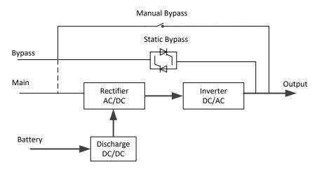
Fig.1-5 Battery mode operation diagram
