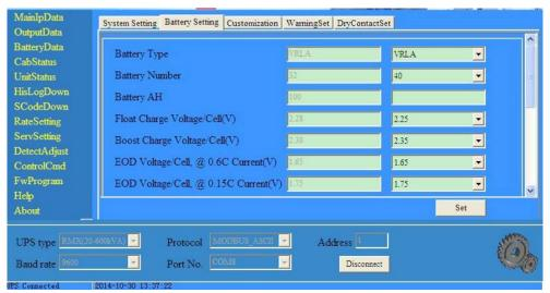
Fig.5-3 Configuration through monitoring software
