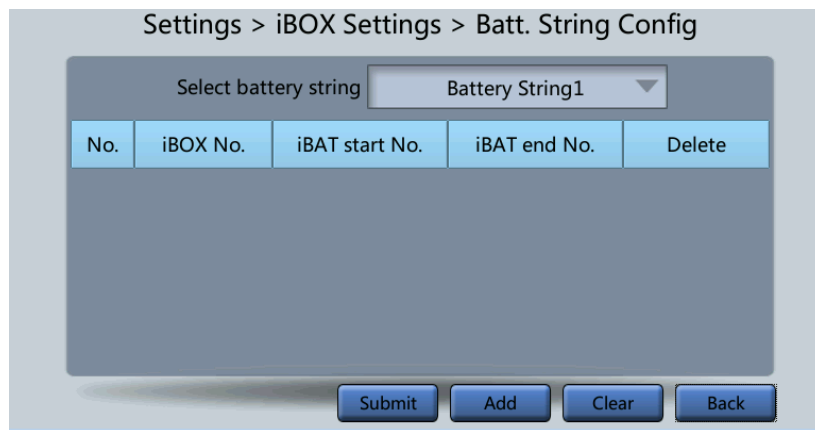
Figure 4-35 Battery string configuration
