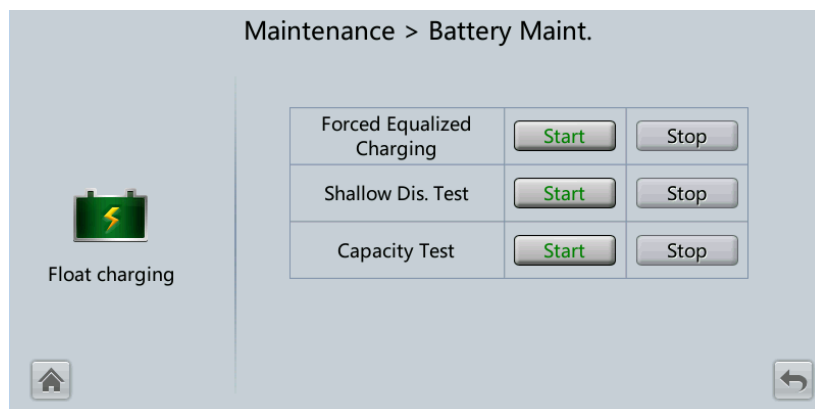
Figure 4-41 Battery maintenance (lead-acid battery)
