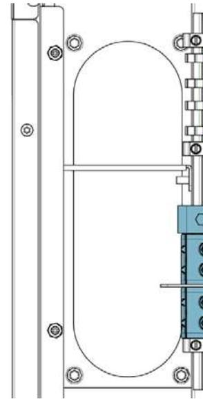
Figure 5. EBC power cable and battery shunt trip cable terminations
